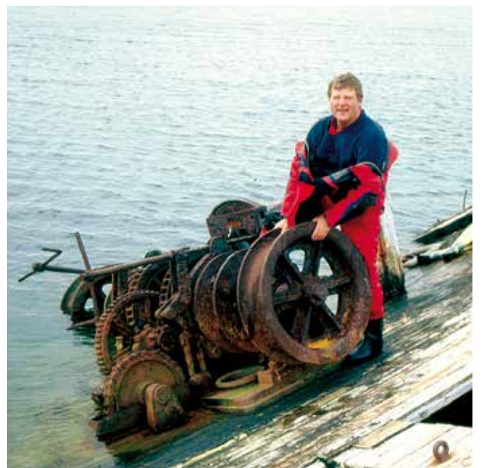
Reference: MacGregor anchor winch on board the wreck of MAUD , Northern Canada.
