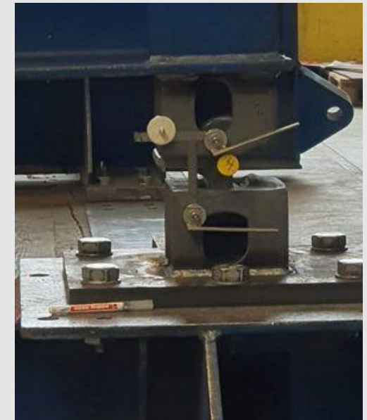
No slip-out with 500kN of lifting force. Compression 350kN, racking force 150kN
