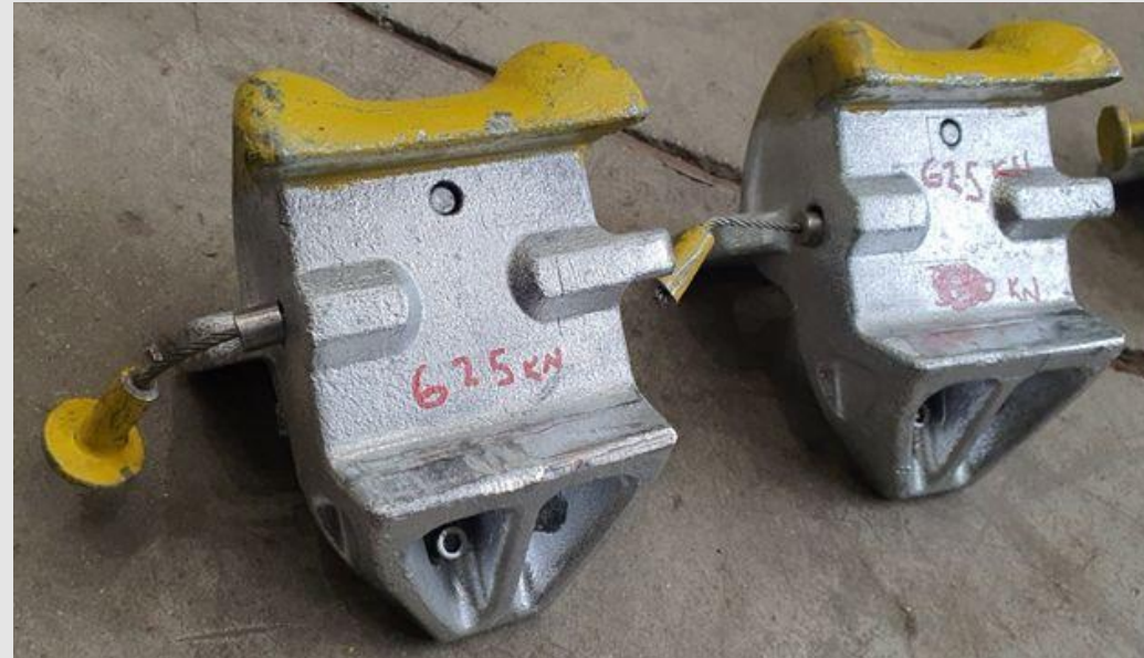
ACV-1's tested to tension of 625kN
