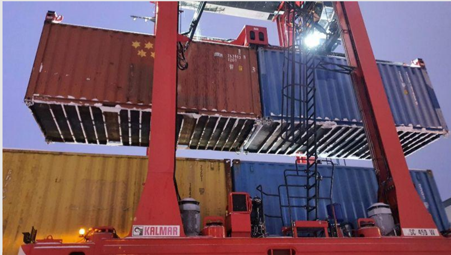
Horizontal tandem lifting of 20ft containers = OK
