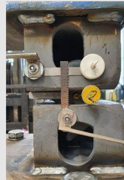
Vertical clearance less than 12mm at SWL lifting force of 250kN
